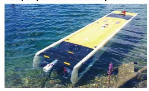
tilising robots to perform inspection of renewable energy plants' critical underwater assets might sound complex. But advances in Remotely Operated Vehicle (ROV) technology have allowed Hibbard Inshore to inspect underwater hydropower structures with less risk, while often reducing overall project costs.
